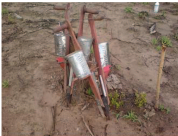
Fig. 18.2 Mechanical jab planters for manual direct seeding and fertilizer application
