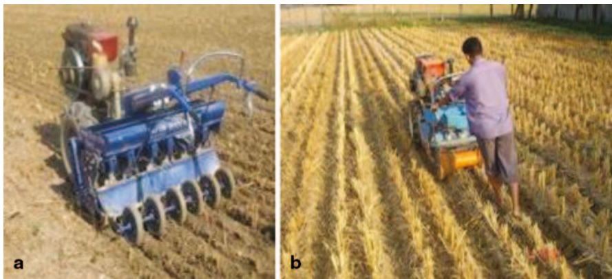
Fig. 5.11 a Strip-tillage-based drill and b bed reshaper/strip-till
