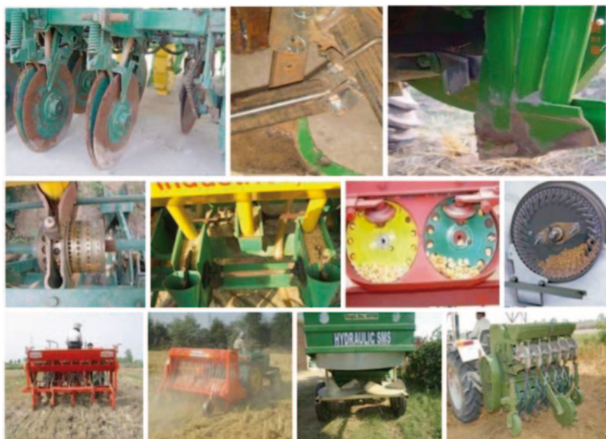
Fig. 11.2 Prototypes of different conservation agriculture-based drills, planters, and seed metering system
