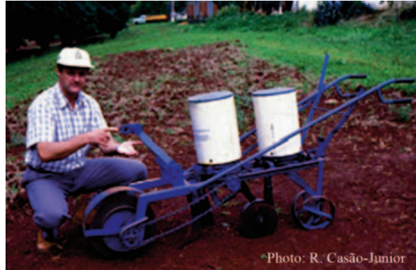
Fig. 16.2 An animal-powered no-till seeder. (Source: Casão-Junior et al. 2012)
